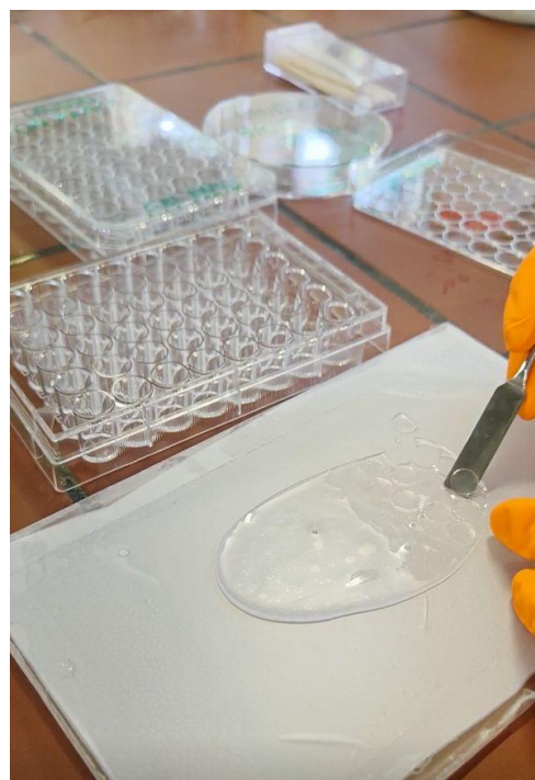
Preparation of a hydrogel swellability/swelling test. Source: 4Tissue
